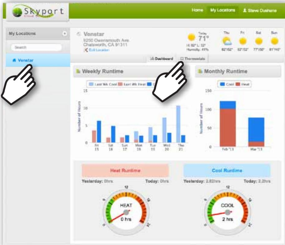
Skyport allows you to monitor room air temperature, supply air temperature and troubleshoot HVAC units remotely. First, highlight the Location and then click "Thermostats"
