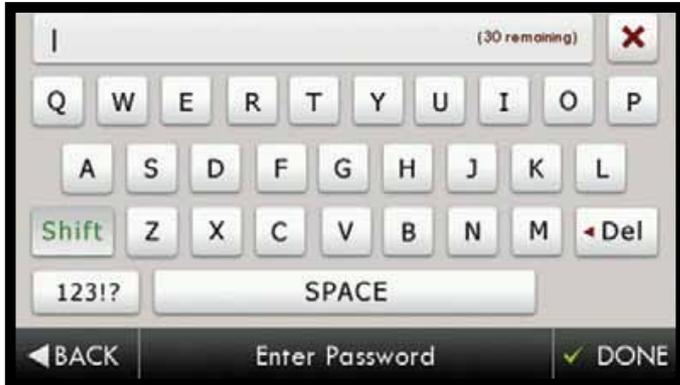
If the network requires security, press **PASSWORD** and enter the password on the keyboard, then press **DONE**. If no security is required, **PASSWORD** will not appear. Press **NEXT** to continue.
