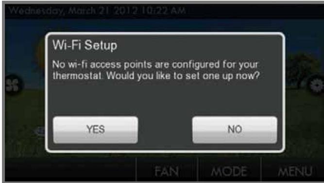
When the Wi-Fi Key is successfully detected this screen will appear.
